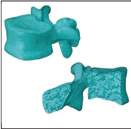
Figure 5. 3D Finite Element Mesh.
